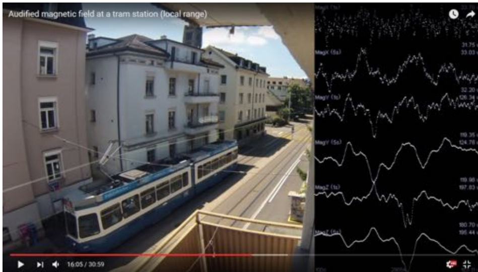
Figure 3. Left: Footage of the actual tram traffic. Right: The recorded magnetic field amplitude at x , y and z axes for two moving average windows of 1 and 5 seconds.
