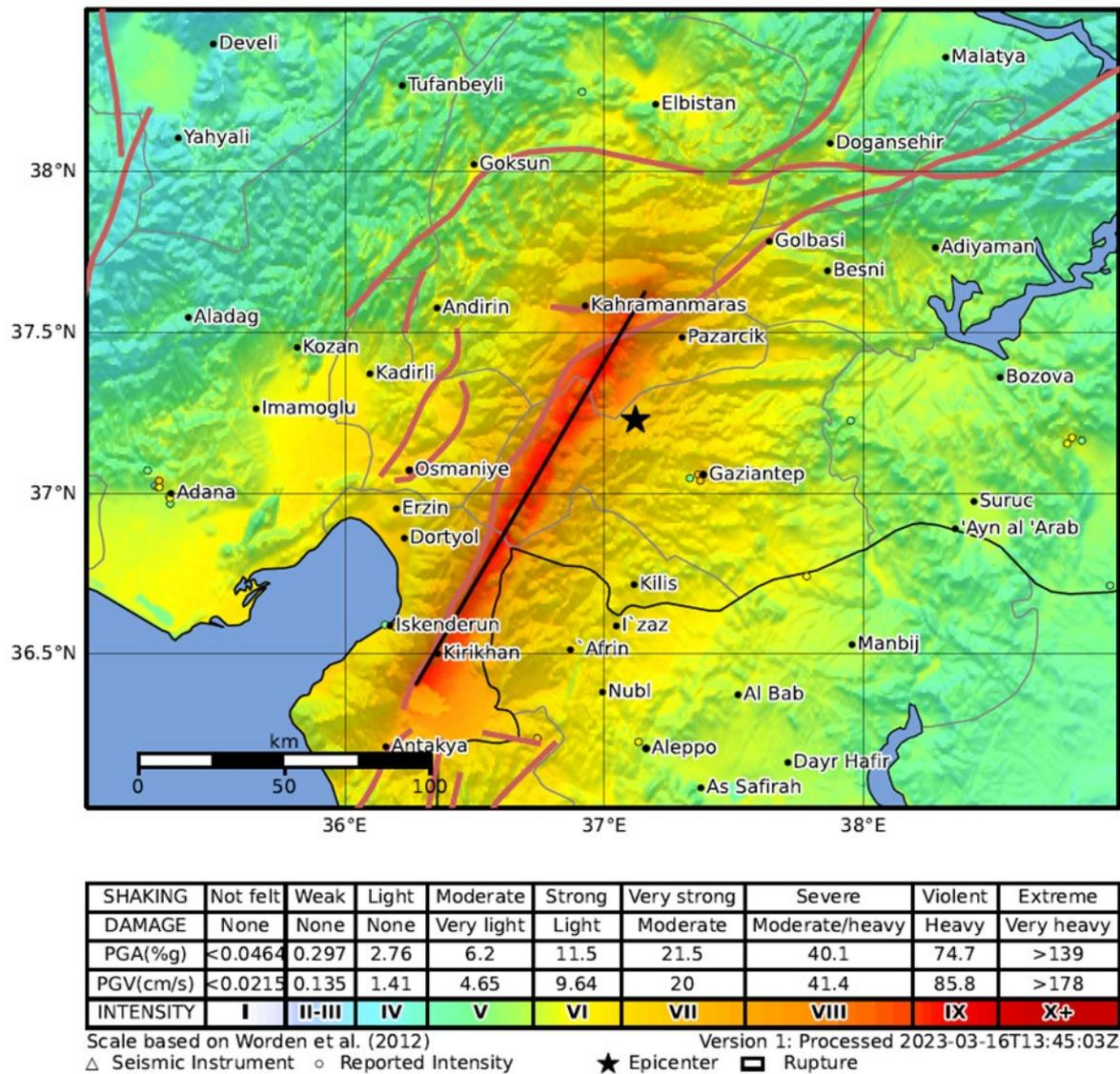
**FIGURE 7 : FAULT GEOMETRY (BLACK LINE) DETERMINED FROM THE ANALYSIS OF FELT REPORTS COLLECTED WITHIN 10 MINUTES OF THE EARTHQUAKE. THE GEOMETRY IS THEN USED AS THE SEISMIC SOURCE TO RECALCULATE THE EXPECTED SPATIAL DISTRIBUTION OF SHAKING AND DAMAGE WHICH AGREES WELL WITH THE OBSERVED DAMAGE (FIGURE 5).**
