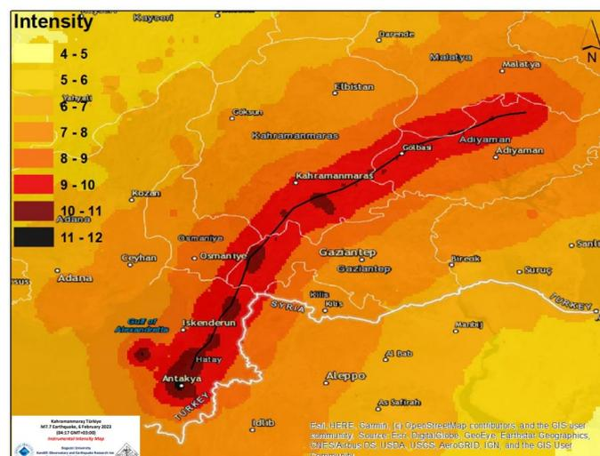
**FIGURE 6 :** FAULT RUPTURE (BLACK LINE) AND DAMAGE LEVEL FROM FIELD SURVEY. THE RUPTURE HAS A LENGTH OF 300 KM.
