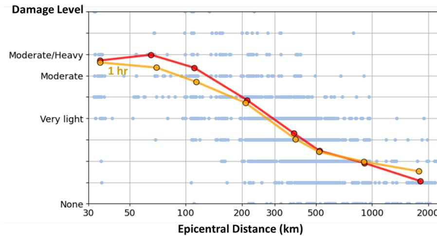
**FIGURE 5 :** INTENSITY CURVES AS A FUNCTION OF EPICENTRAL DISTANCE ARE AUTOMATICALLY DETERMINED FROM INDIVIDUAL FELT REPORTS (BLUE DOTS). THE MAXIMUM INTENSITY DETERMINED AFTER ONE HOUR (ORANGE CURVE) UNDERESTIMATES THE FINAL VALUE (RED CURVE).
