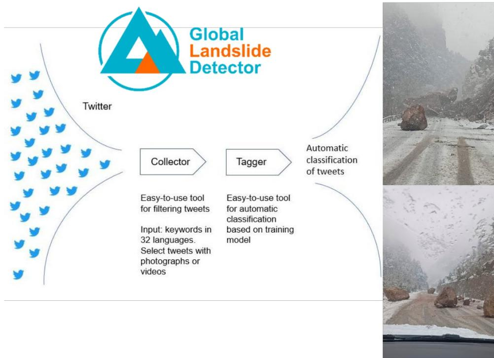
**FIGURE 9 :** THE GLOBAL LANDSLIDE DETECTOR COLLECTS TWEETS MENTIONING “LANDSLIDE” IN DIFFERENT LANGUAGES, THEN A MANUALLY TRAINED ARTIFICIAL INTELLIGENCE ENGINE REJECTS IMAGES NOT RELATED TO LANDSLIDES. A TRIGGERED LANDSLIDE (RIGHT IMAGES) WAS DETECTED 12 HOURS AFTER THE KAHRAMANMARAŞ EARTHQUAKE.
